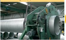
Machining the bevel prepares the pipe-ends for circumferential welding
