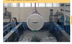
All corrosion resistant pipes are full body pickled at BUTTING
