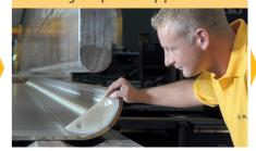
Press brakes and a three-roller bending machine are available to form the plates
