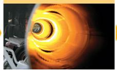
The pipes are annealed both in the furnace and inductively
