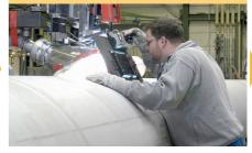
Pipes with an outside diameter of up to 2 032 mm can be connected into max. 24-m lengths by circumferential welding
