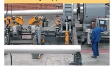
In this stage of production, the pipe ends can be bevelled or faced
