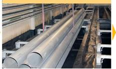
At BUTTING, all pipes are full body pickled – this results in a passive layer to protect against corrosion
