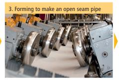
The coil is formed into an open seam pipe by means of profiling rollers
