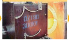
Heat treatment is performed online – in an inductive solution annealing process followed by a rapid cooling
