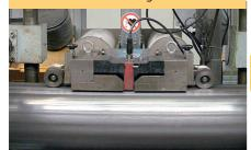
A leakage test of the longitudinal weld is performed online; the equipment highlights any faulty areas
