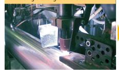
The longitudinal seam is welded using the laser beam, plasma or TIG welding process
