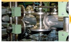
The pipes are calibrated in line with the tolerance requirements
