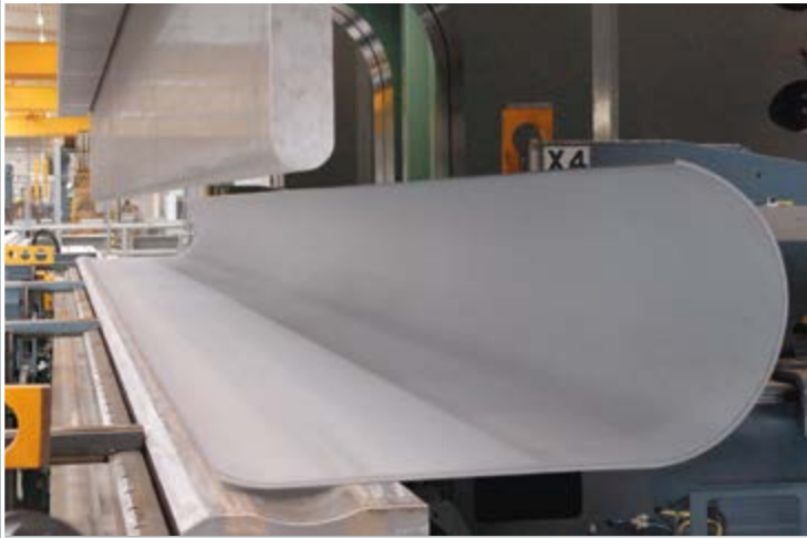
Plates are edged or formed and then welded into pipes
