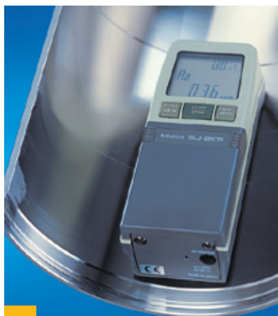
Roughness measurement of inside surface of longitudinally welded pipes
